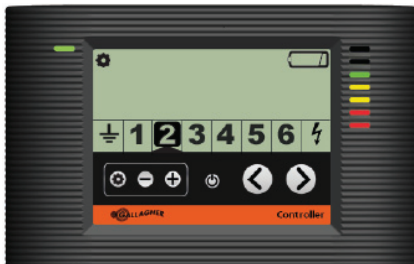
Bedieningspaneel toont zone 2 met lege batterijen
