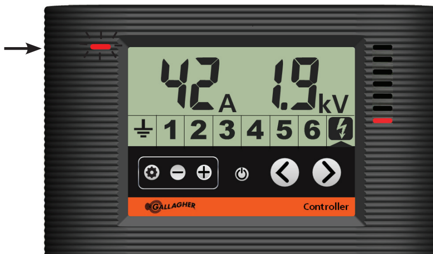
Controller showing the energizer in output alarm
