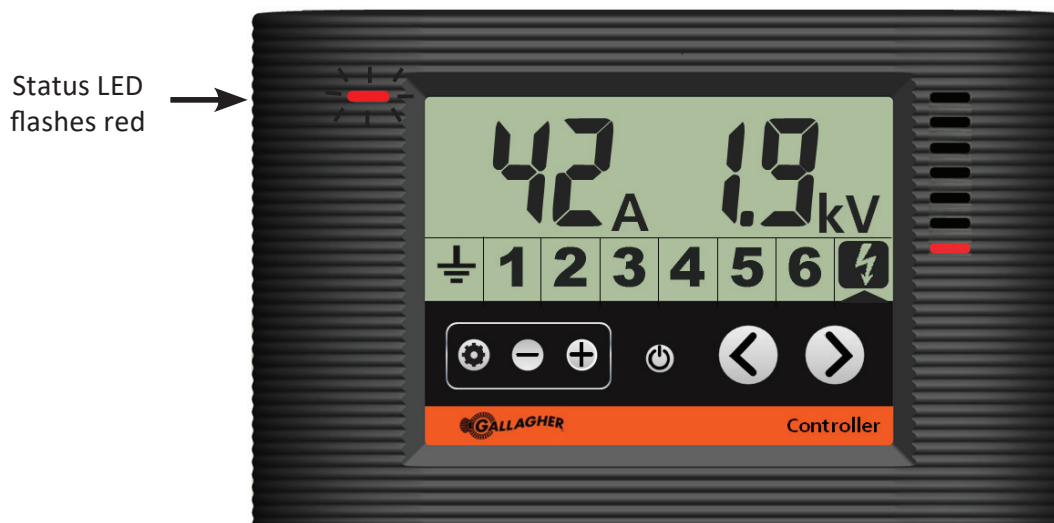
Controller showing the energizer in output alarm
