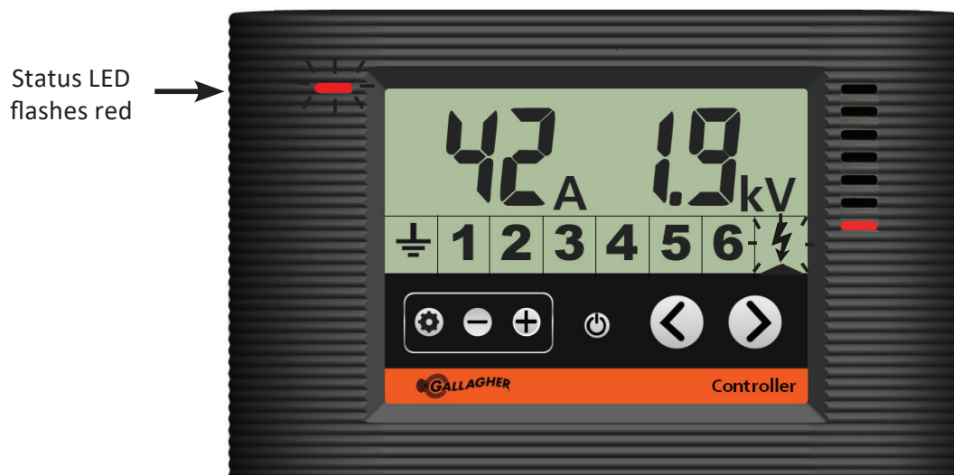
Controller showing the energizer in current alarm
