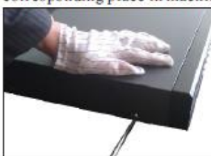
6. Fix the screws of the top cover .
