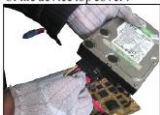
3. Connect hard disk power line
