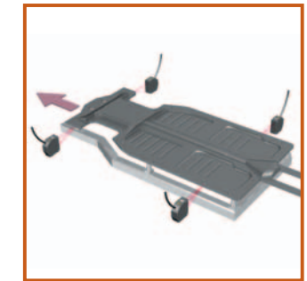
Measuring Car Body Widths (ZS-HLDS10)
