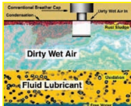
An illustration showing what a reservoir without an Ultra Clean Contamination Control Breather looks like.
